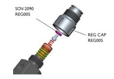
Then ease the cap down over the bobbin assembly ensuring the O ring Reg 060 enters the bore without damage or nicking. Once fully over the bobbin some green high strength thread locking compound can be applied to the thread and the cap screwed down. The cap can then be tightened down with a "C" spanner (Gedore No.40), the grub screw Reg 070 is then screwed in using a 1/16th allen key.
